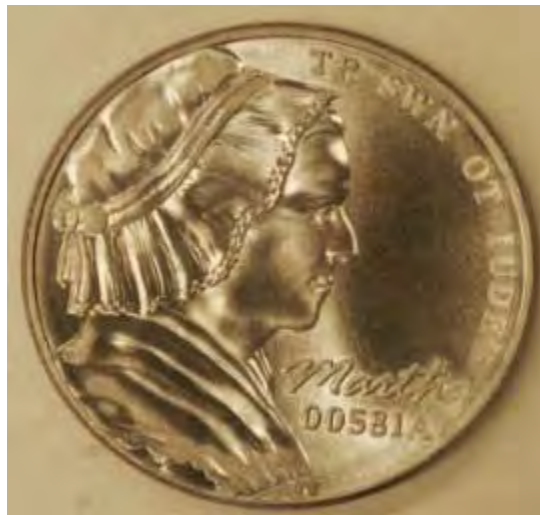
Figure 2-8. 430 stainless steel 5-cent nonsense piece struck at 70 tonnes.
