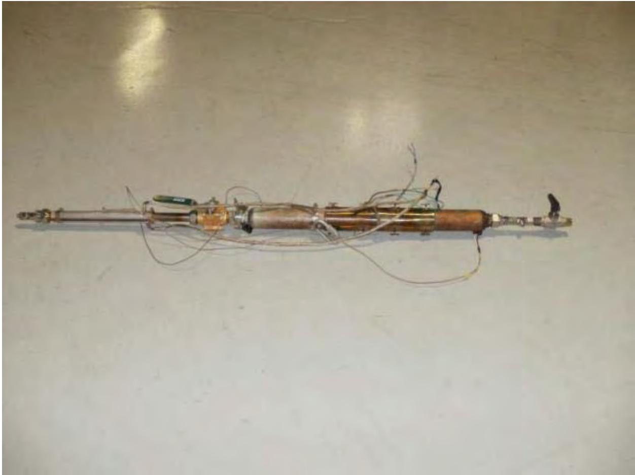
Figure 2-G-16.CVMR prototype carbonyl reactor.
