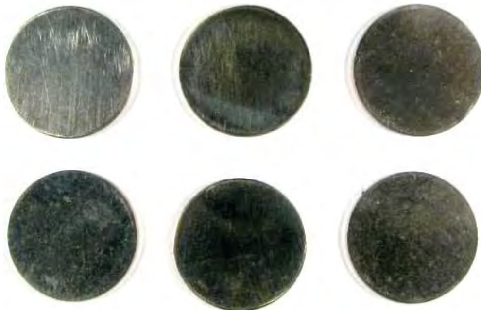
Figure 2-D-18. Steam corrosion tested incumbent dollar coin planchets.
