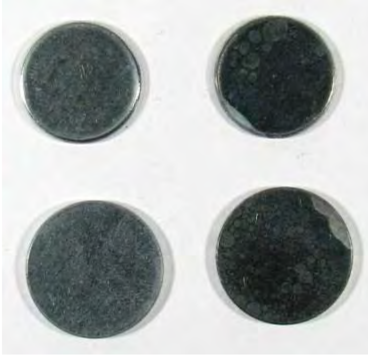
A26-coated one-cent blanks (top) and B21-coated 5-cent blanks (bottom). Figure 2-G-3. Coated A190 plachets as-coated (left) and after steam corrosion testing (right).
