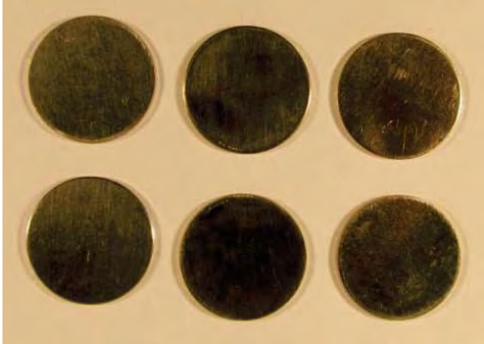
Figure 2-D-20. Steam corrosion tested K474 copper alloy dollar blanks.
