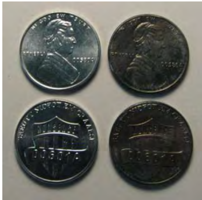
Figure 2-G-4. A26-coated A190 one-cent nonsense pieces before (left) and after (right) steam corrosion testing.
