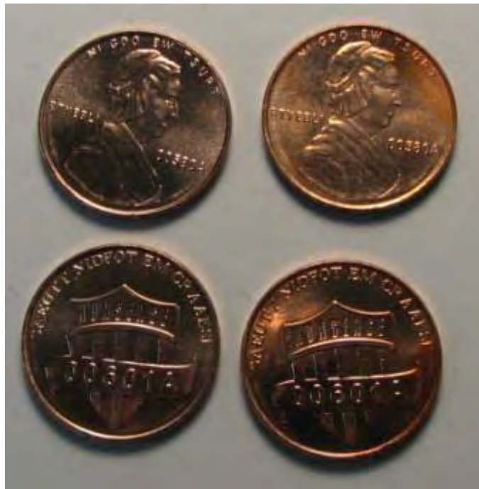
Two pieces on left are as-struck and two on right are after a 2-hour steam corrosion test. Figure 2-E-3. Steam corrosion tested copper-plated steel (Royal Mint) one-cent nonsense pieces.
