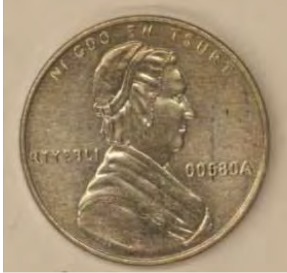
Figure 2-12. 5052-H32 one-cent nonsense piece struck at 25 tonnes.
