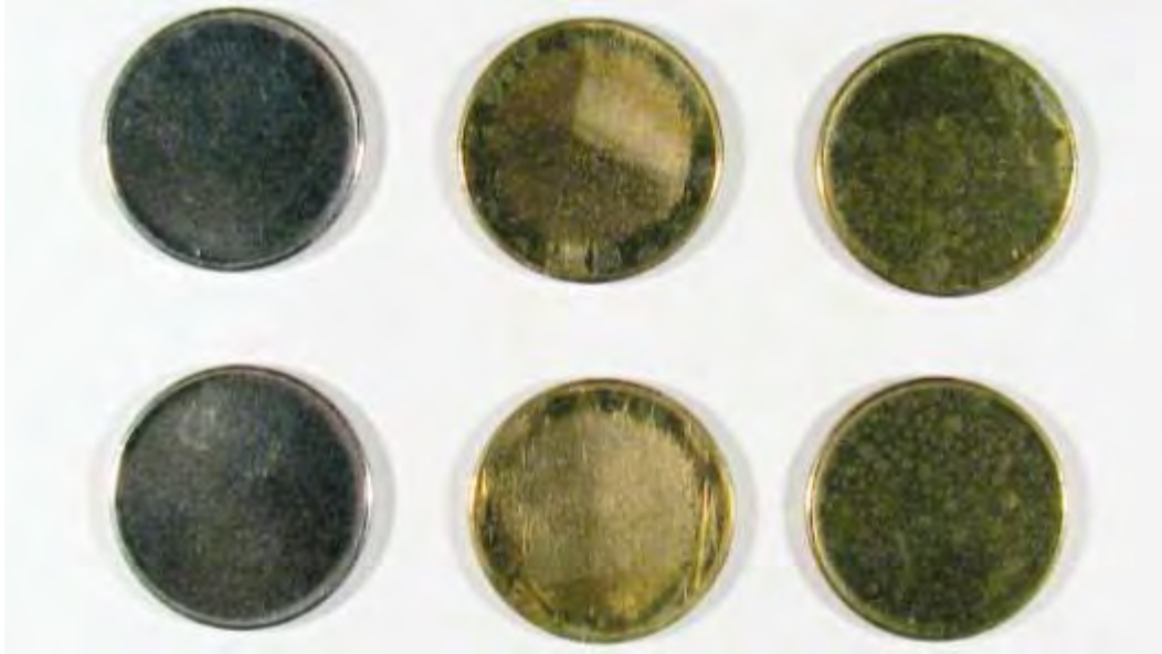
Nickel-plated surface after corrosion test on left, unplated, lightly sanded surface after test in middle, and unplated ready-to-strike after corrosion test on right.
