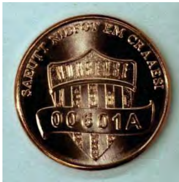
Figure 2-3. JZP copper-plated steel one-cent nonsense piece struck at 40 tonnes.
