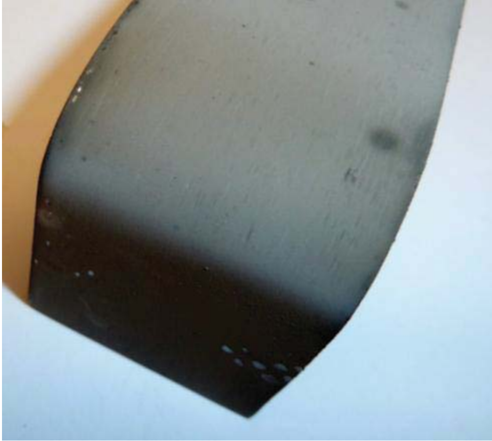
Figure 2-G-11. Carbonyl nickel-coated steel specimen after single-bend testing.
