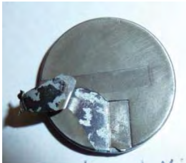
Figure 2-G-10. Carbonyl nickel-coated zinc surface after hammer indent testing.
