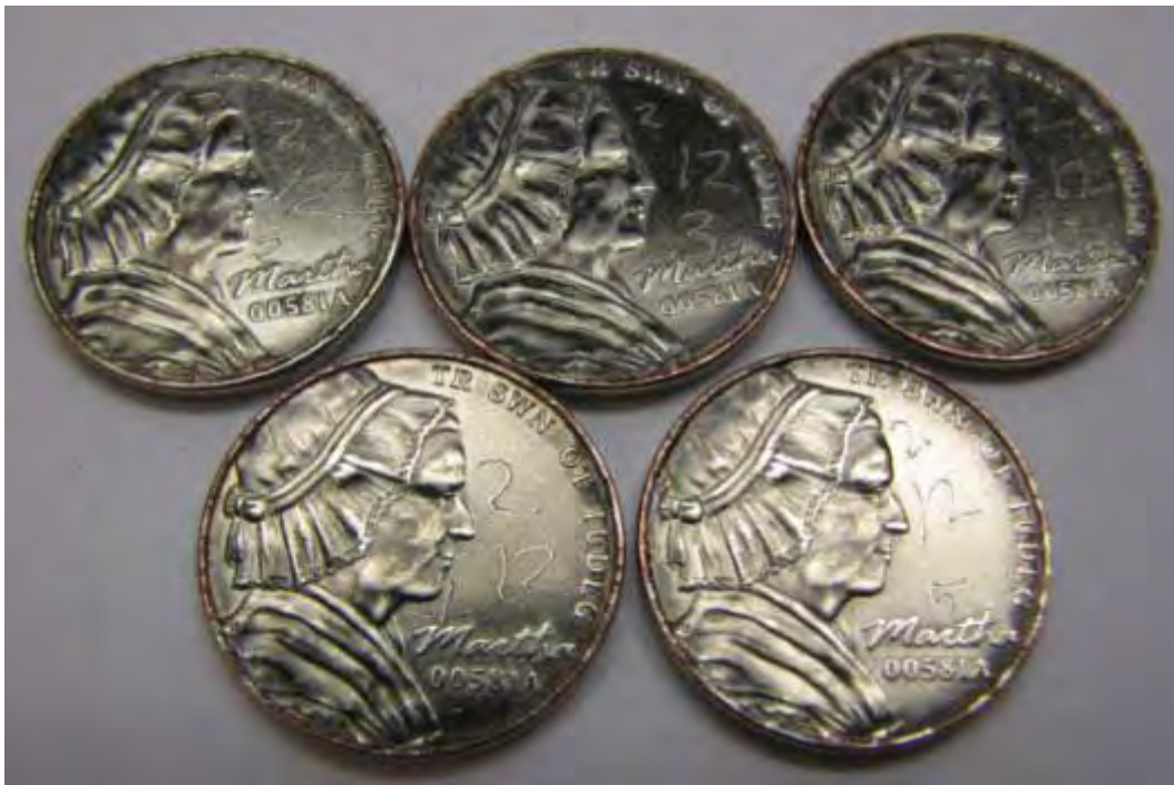
Figure 2-F-10. Wear tested Multi-Ply-plated steel 5-cent nonsense pieces.
