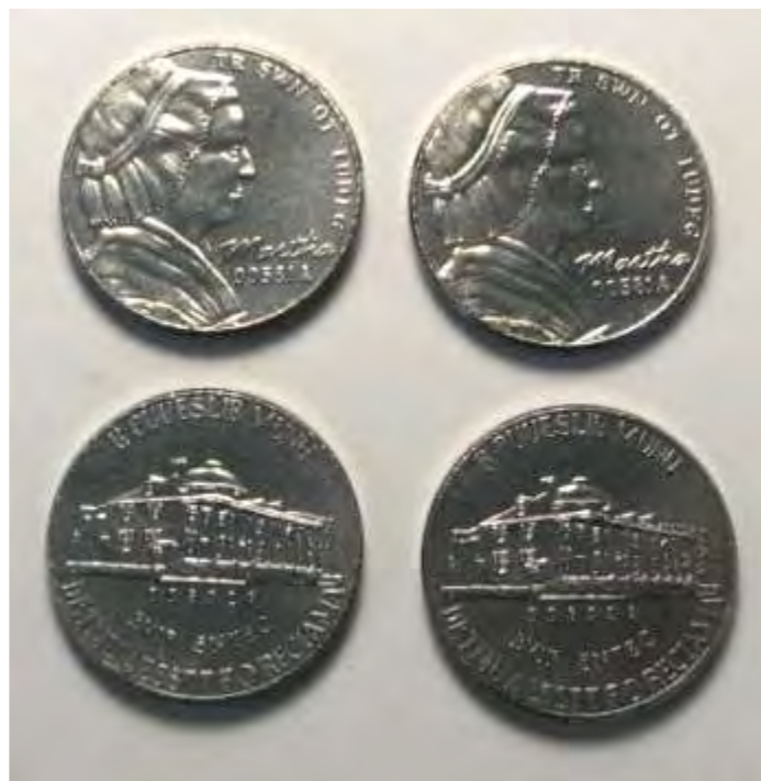
Figure 2-E-14. Steam corrosion tested 430 stainless steel 5-cent nonsense pieces.
