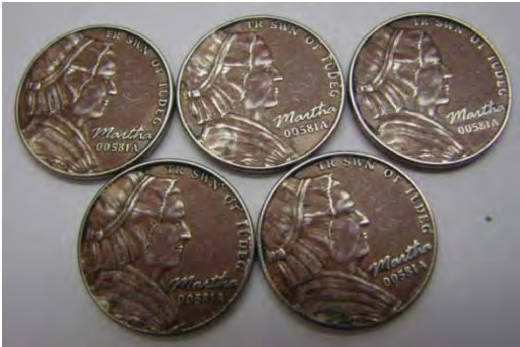
Figure 2-F-8. Wear tested 5-cent nonsense pieces (incumbent material).
