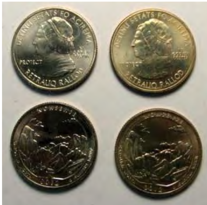
Two pieces on left are as-struck and two on right are after a 2-hour steam corrosion test. Figure 2-E-21. Steam corrosion tested 669z-clad C110 quarter dollar nonsense pieces.
