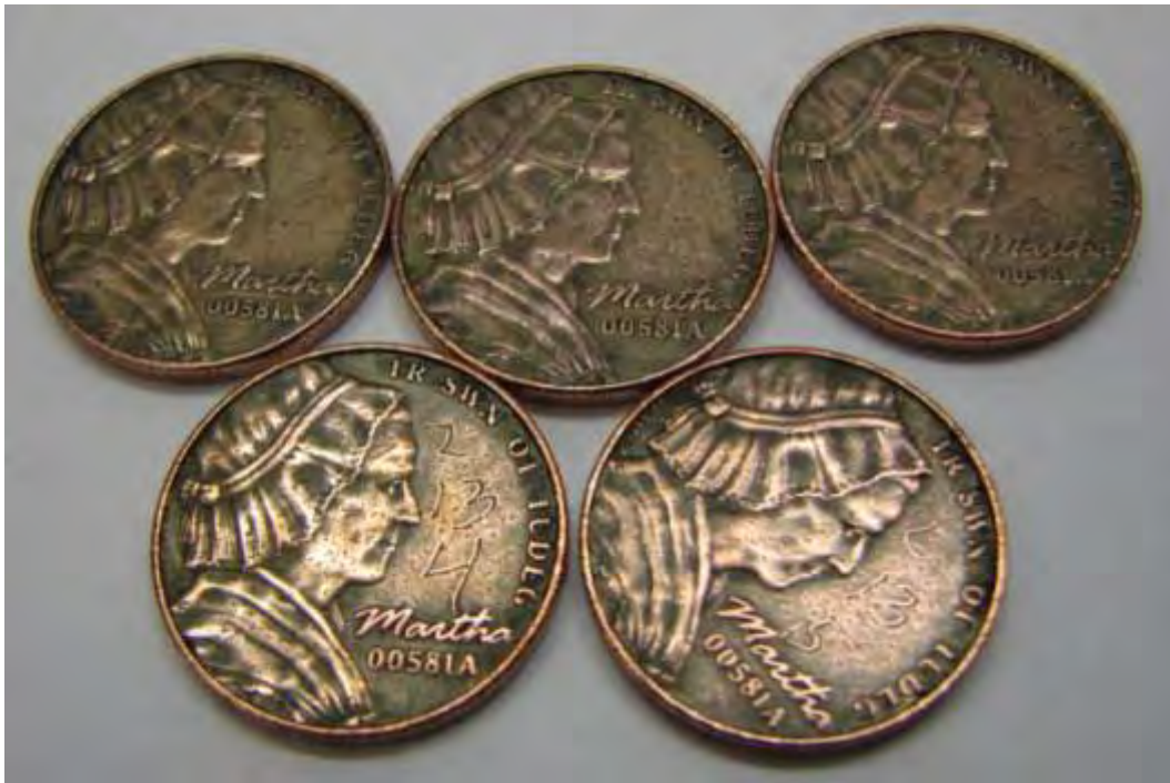
Figure 2-F-16. Wear tested nickel-plated 31157 5-cent nonsense pieces.
