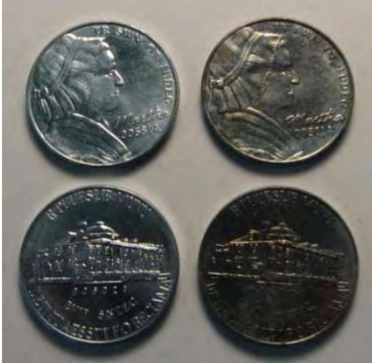
Figure 2-G-5. B21-coated A190 5-cent nonsense pieces before (left) and after (right) steam corrosion testing.
