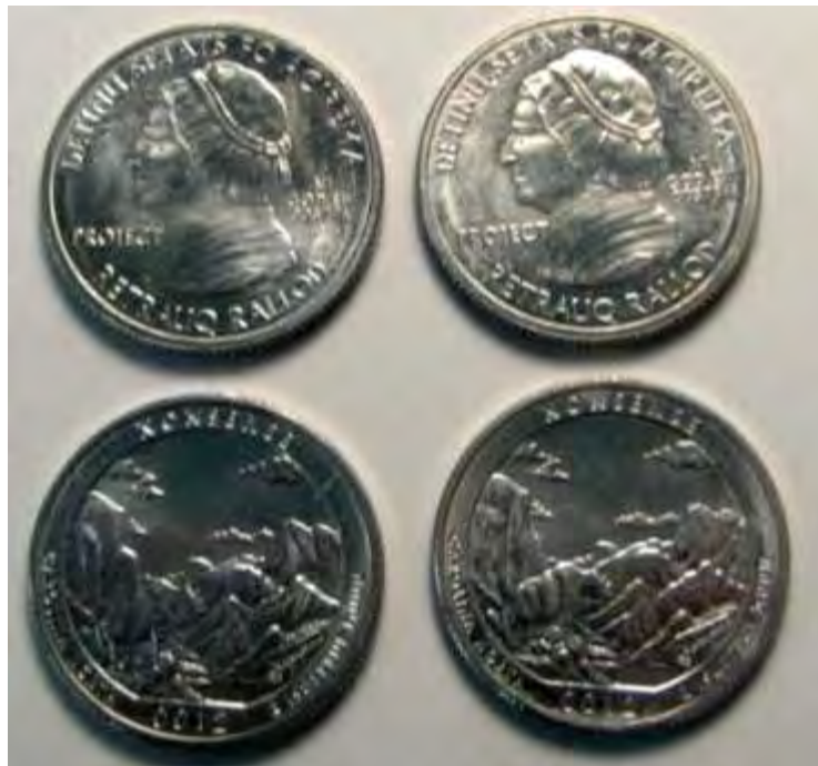
Two pieces on left are as-struck and two on right are after a 2-hour steam corrosion test. Figure 2-E-23. Steam corrosion tested Dura-White-plated zinc quarter dollar nonsense pieces.
