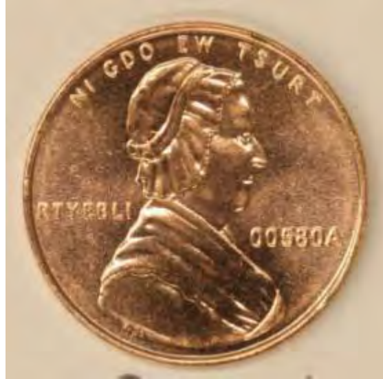
Figure 2-13. Copper-plated steel one-cent nonsense piece struck at 50 tonnes from planchets supplied by the Royal Mint.
