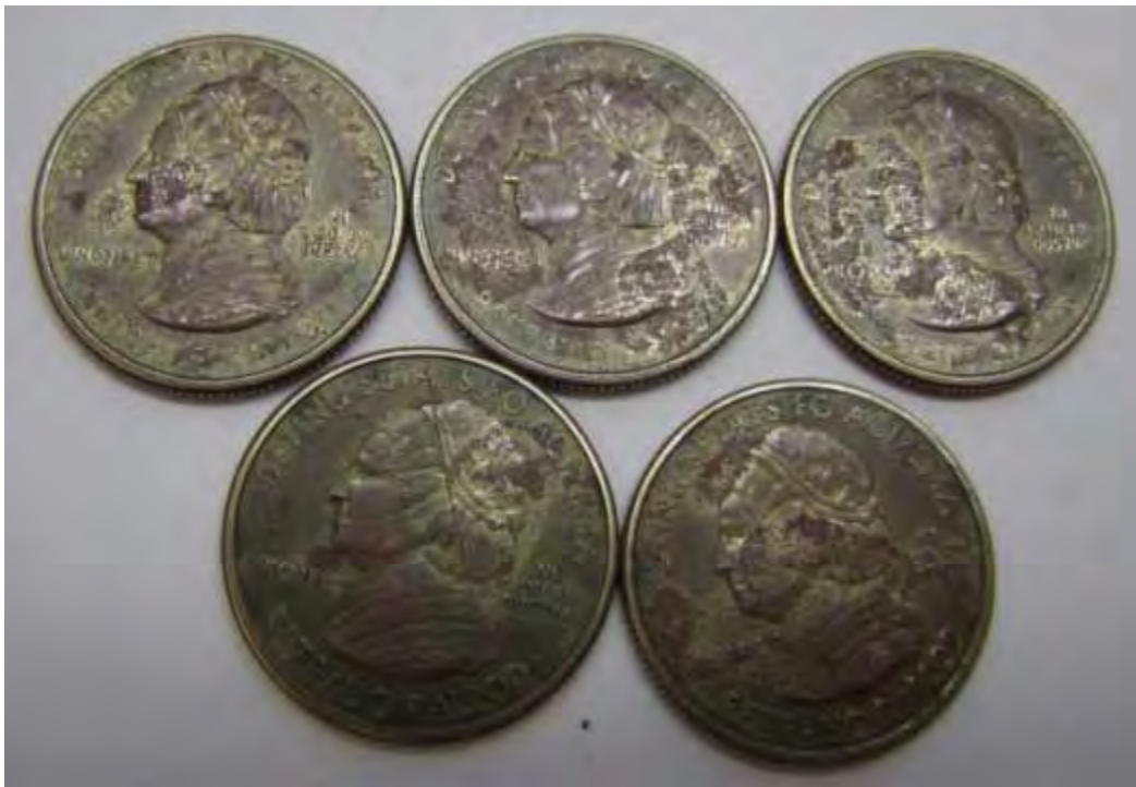
Figure 2-F-20. Wear tested nickel-plated steel quarter dollar nonsense pieces.
