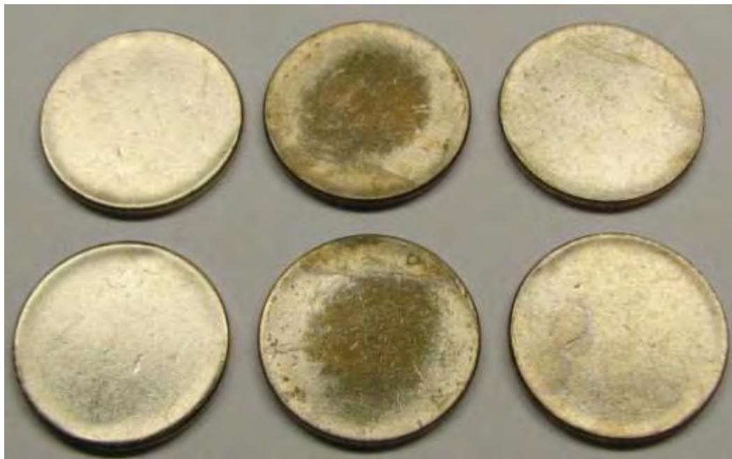
Untested, as-received on left, lightly sanded and tested in middle, and tested in ready-to-strike condition on right.
