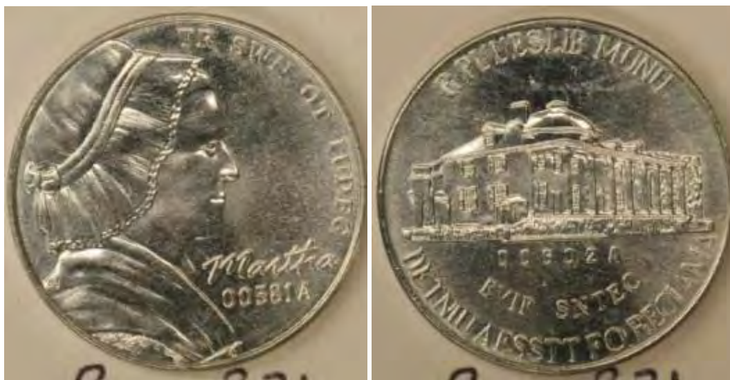
Figure 2-G-2. B21-coated A190 5-cent nonsense piece struck at 54 tonnes.
