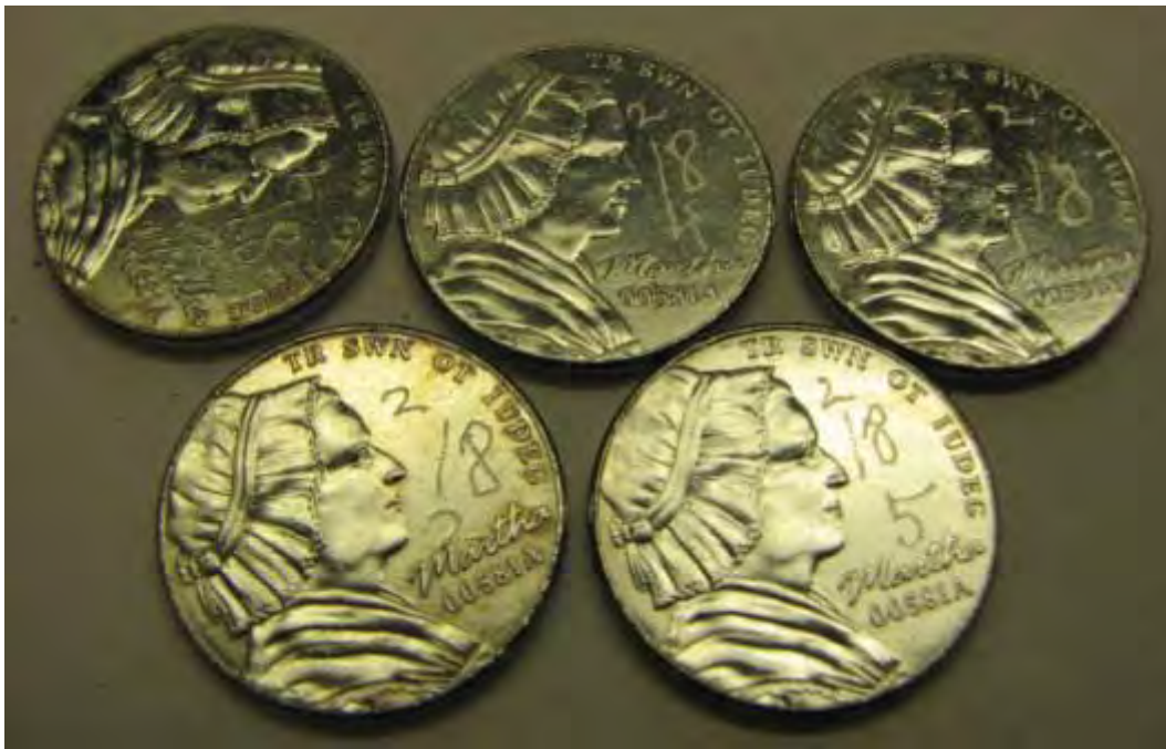
Figure 2-F-14. Wear tested 430 stainless steel 5-cent nonsense pieces.
