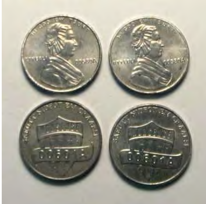
Figure 2-E-4. Steam corrosion tested 5052-H32 one-cent nonsense pieces.
