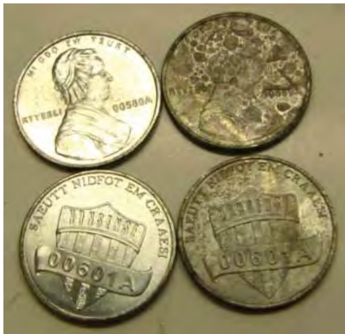
Figure 2-E-4. Steam corrosion tested 5052-H32 one-cent nonsense pieces.
