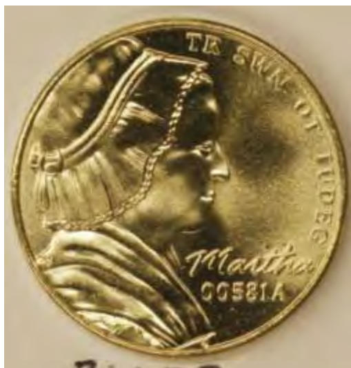
Figure 2-18. Unplated 31157 5-cent nonsense piece struck at 54 tonnes.
