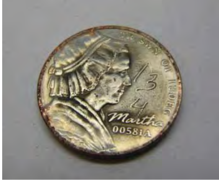
Figure 2-F-16. Wear tested nickel-plated 31157 5-cent nonsense pieces.
