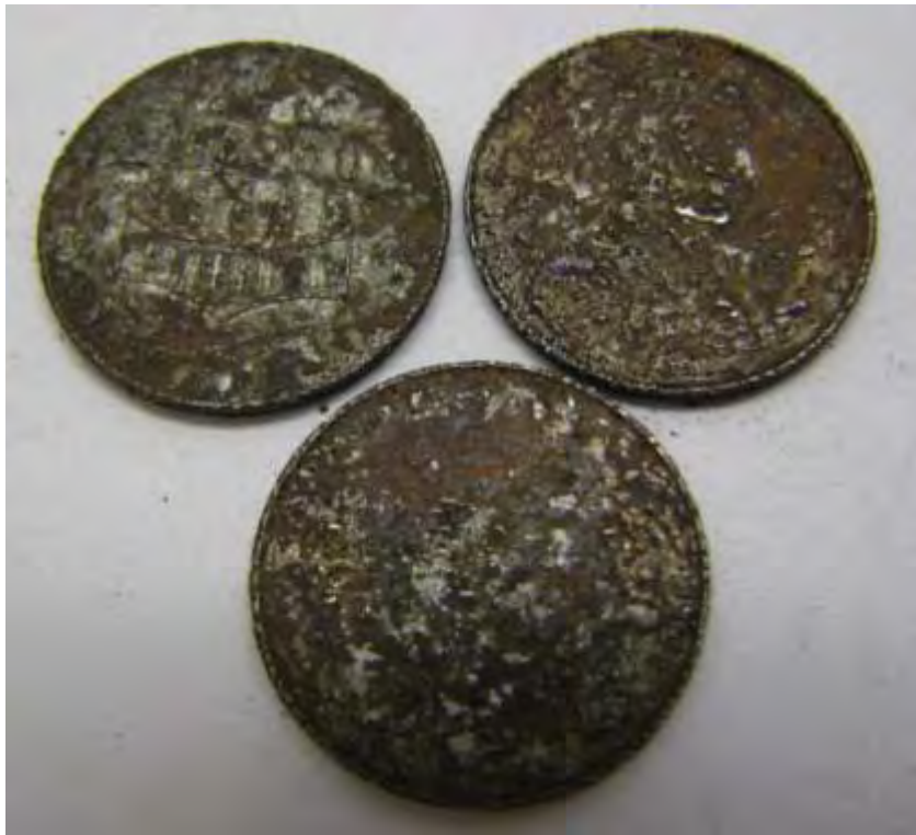
Figure 2-F-4. Wear tested 5052-H32 one-cent nonsense pieces.
