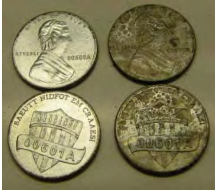
Two pieces on left are as-struck and two on right are after a 2-hour steam corrosion test. Figure 2-E-6. Steam corrosion tested aluminized steel (Ryerson) one-cent nonsense pieces.
