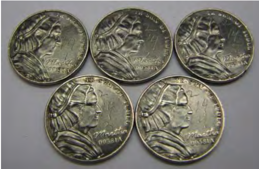
Figure 2-F-10. Wear tested Multi-Ply-plated steel 5-cent nonsense pieces.
