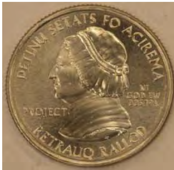
Figure 2-9. 669z-clad C110 quarter dollar nonsense piece struck at 62 tonnes.
