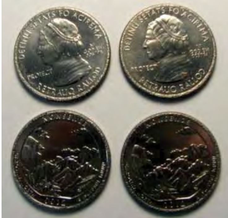
Two pieces on left are as-struck and two on right are after a 2-hour steam corrosion test. Figure 2-E-22. Steam corrosion tested 302HQ stainless steel quarter dollar nonsense pieces.
