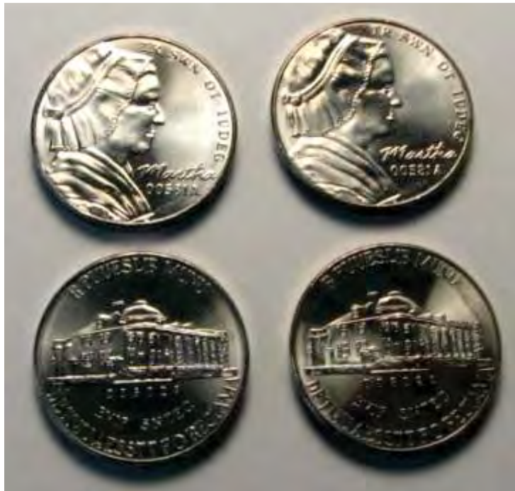
Two pieces on left are as-struck and two on right are after a 2-hour steam corrosion test. Figure 2-E-11. Steam corrosion tested nickel-plated steel 5-cent nonsense pieces.
