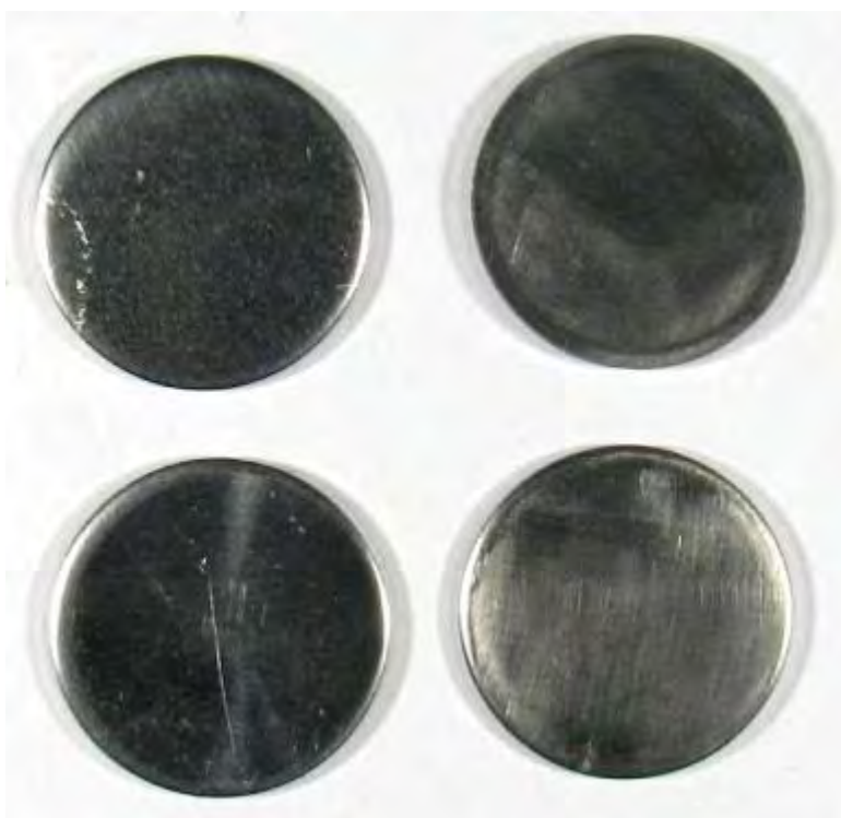
Figure 2-D-12.Steam corrosion tested 430 stainless steel 5-cent blanks.
