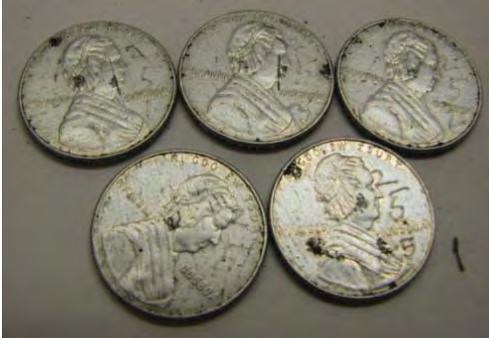
Figure 2-F-4. Wear tested 5052-H32 one-cent nonsense pieces.
