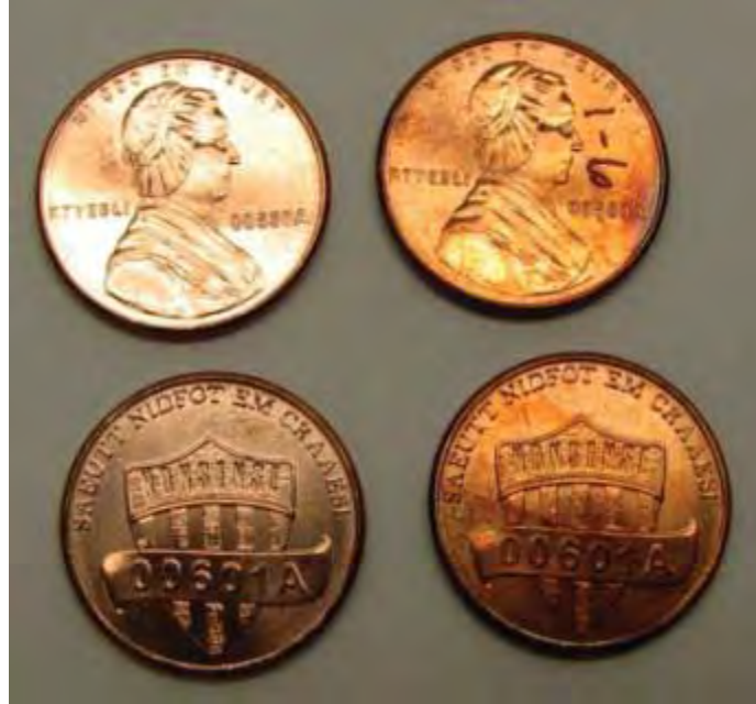
Two pieces on left are as-struck and two on right are after a 2-hour steam corrosion test. Figure 2-E-2. Steam corrosion tested copper-plated steel (Jarden Zinc Products) one-cent nonsense pieces.
