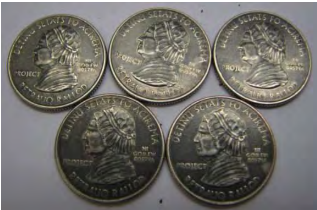
Figure 2-F-18. Wear tested quarter dollar nonsense pieces (incumbent material).
