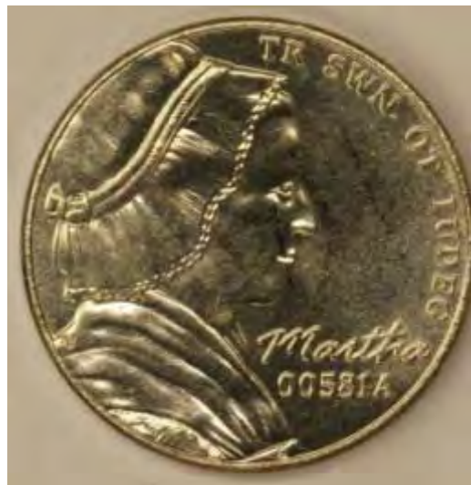
Figure 2-16. G6 mod 5-cent nonsense piece struck at 54 tonnes.
