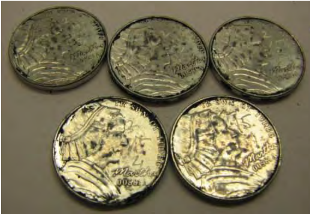
Figure 2-F-8. Wear tested 5-cent nonsense pieces (incumbent material).
