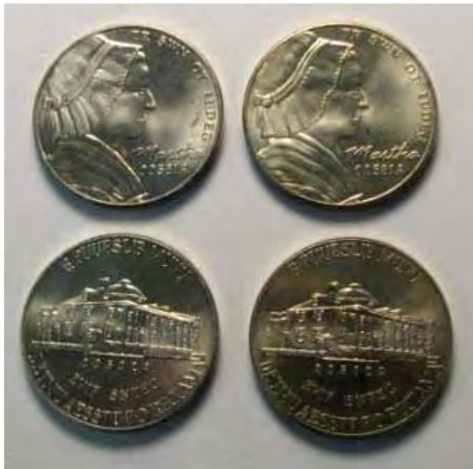
Figure 2-E-12. Steam corrosion tested G6 mod 5-cent nonsense pieces.
