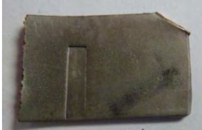
Figure 2-G-9. Carbonyl nickel-coated zinc surface after hammer indent testing with a steel punch.
