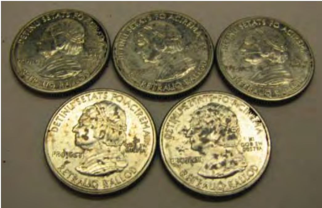
Figure 2-F-22. Wear tested 302HQ stainless steel quarter dollar nonsense pieces.
