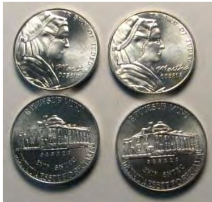
Figure 2-E-8. Steam corrosion tested 5-cent nonsense pieces (incumbent material).
