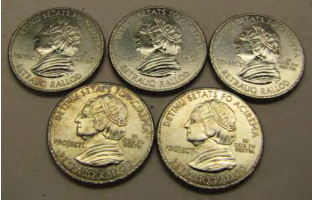
Figure 2-F-22. Wear tested 302HQ stainless steel quarter dollar nonsense pieces.
