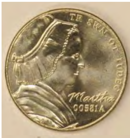
Figure 2-17. 669z 5-cent nonsense piece struck at 54 tonnes.
