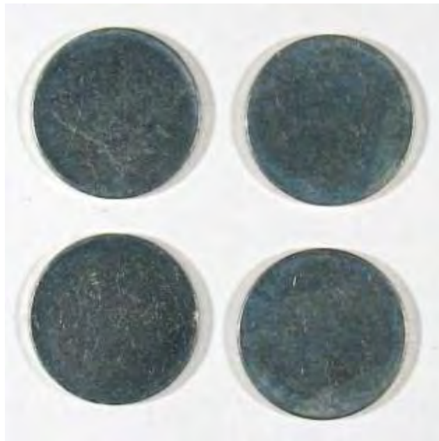
Figure 2-D-6. Steam corrosion tested cupronickel 5-cent planchets (incumbent US 5-cent coin material).
