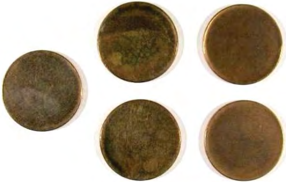
Untested, as-received on left, lightly sanded and tested in middle, and tested blanks on right. Figure 2-D-22. Steam corrosion tested yellow bronze- (88Cu-12Sn-) plated zinc dollar blanks.
